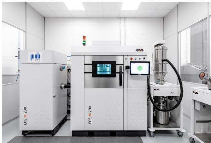
① Construction volume is 250x250x300 mm
